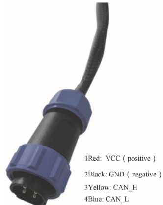
Figure 3.2 Schematic diagram of aviation plug male
