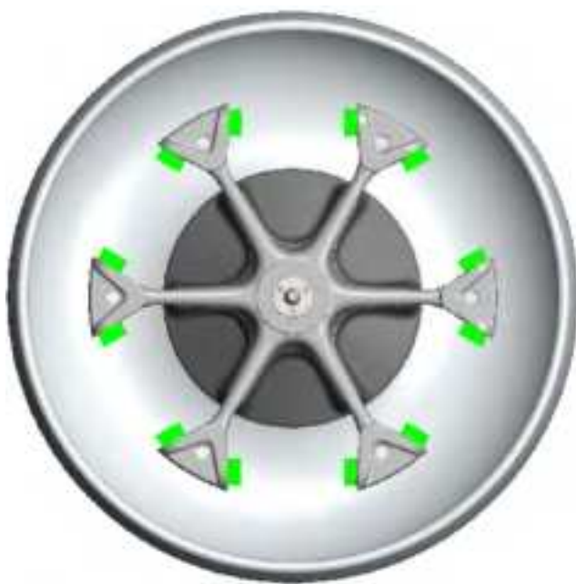
Figure III-7: Lubricate trunnion bolts, e.g. HAEMAFlex 12
