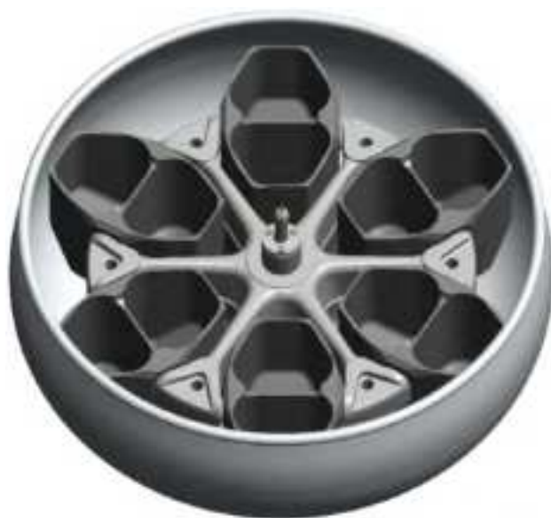
Figure III–8: Install buckets into rotor, e.g. HAEMAFlex 12
