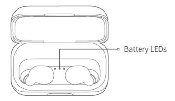
All three battery LEDs will blink 3 times then numbers of them will glow solid for 30s according to practical battery level whenever you open or close lid. (If you need to check battery level again, please close and re-open the lid again.) Low battery warning: only one LED blinks white.
