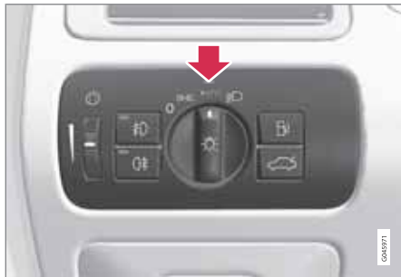
Light switch in the AUTO position
