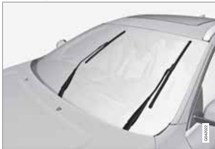
Wiper blades in service position
