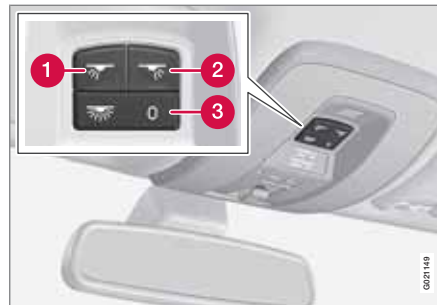
Light switches, front roof lighting
