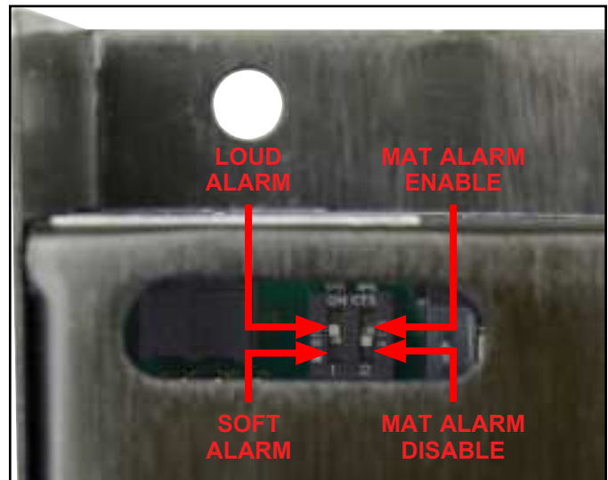
Figure 5. Audible alarm DIP switches located on the bottom side of the 724 Workstation Monitor
