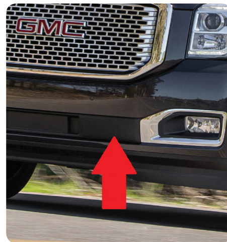
Keep the front fascia clean for proper radar operation.
