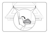
**1.** Open the door and flip open the clips at both hinges.
