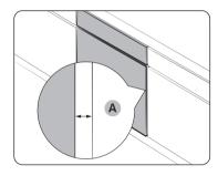
Make sure to leave a gap (A) of at least 5 mm between the oven and each side of the cabinet.
