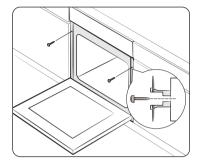
Fit the oven into the cabinet and fix the oven firmly on both sides using 2 screws.
