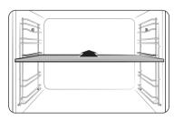
**1.** Insert the Divider in level 3 to separate the cooking chamber in two compartments.
