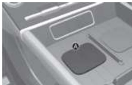
[A] Vehicle authentication pad (wireless charging pad)
