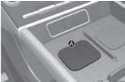
[A] Vehicle authentication pad (Wireless charging pad)
