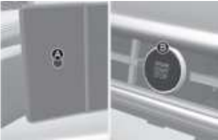
[A] Fingerprint sensor [B] Engine Start/Stop button
