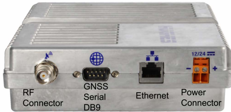
Figure 7: Back side view of IDU
