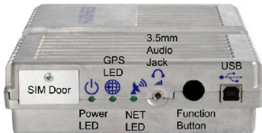
Figure 6: Front side view of IDU
