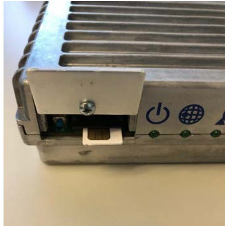
Figure 34: Installing the SIM card
