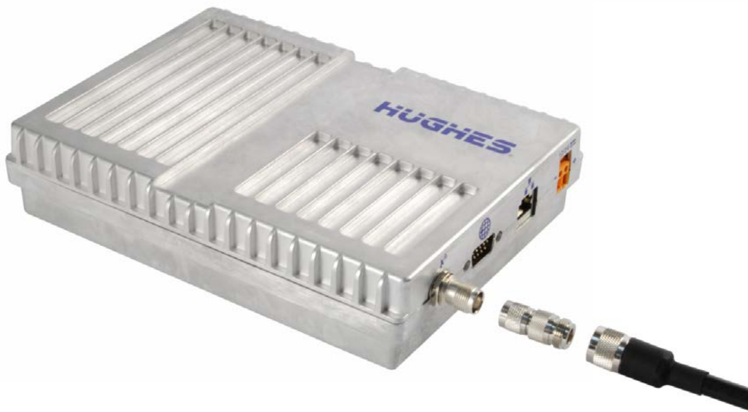
Figure 33: Connect cable to TNC connector on IDU
