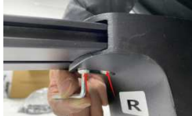
8. Install the crossbars. (Note: Install the longer crossbar towards the front of the vehicle. Once both brackets are in place, tighten the screws to secure the crossbars.)
