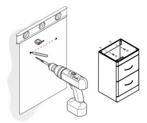
Mark the two holes levelly on the wall.
