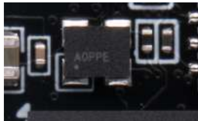
Figure 5-2: 33.333333Mhz active crystal on the core board
