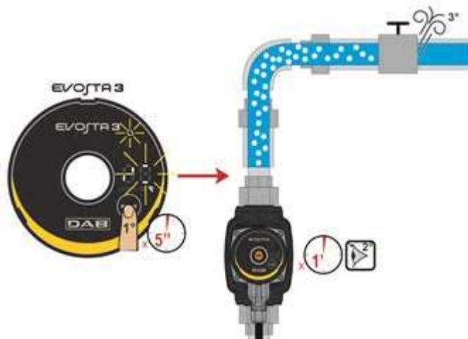
Figure 8: Automatic venting of the pump
