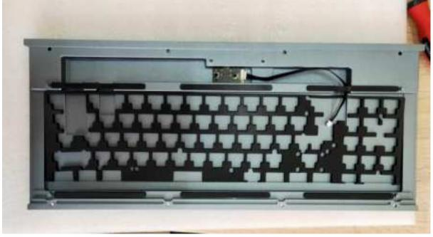
Connect the main PCB with the daughterboard and attach the ffc to the F-row. Place the top case and secure it with M2 black screw\* 8 pcs to complete the assembly. 最後,將主 PCB 與子板連接,並將排線接上 F 排。蓋上上蓋並用 8 顆 M2 黑色螺絲固定,組裝完成。
