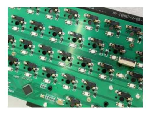
Flip the top case of the kit to the back and position the Poron plate foam, followed by the Poron switch pad along the F-row. Finally, place the PCB on top. Then screin the M2 black screw\*4 pcs.將套件的上蓋翻轉至背面·接著在 F-row 那一排放置 Poron 夾層泡綿和 Poron 軸下墊·最後再放上 PCB。接著再鎖上 4 顆 M2 黑色螺絲將其固定
