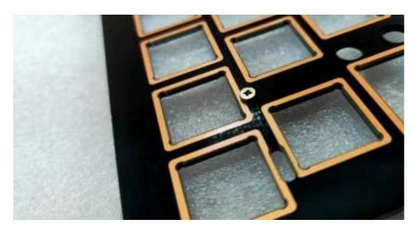
Place the poron switch pad and poron plate foam sequentially onto the PCBA, with the Poron switch pad positioned first, followed by the Poron plate foam.
