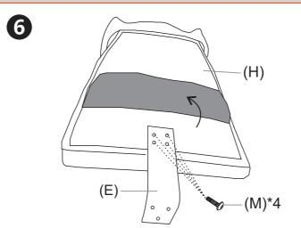
Note: Lift the velcro strips on the back of the Backrest(H), then you will find the screw holes
