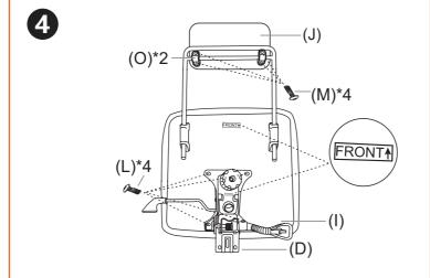
Note: Make sure the "FRONT" markings of the Mechanism (D) and the Seat (I) are in the same direction.
