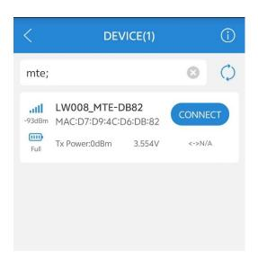
After the device is turned on, the device Bluetooth will start broadcasting. Open the MKLoRa APP and choose LW008, then you can search the LW008-MTE device by click the refresh icon. The default broadcast name of the device: LW008-MTE -XXXX.
