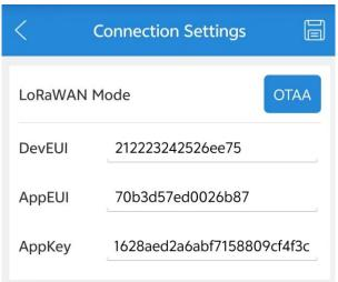
Configure/Read the LoRaWAN mode and the key parameters, such as DevEUI, AppEUI and AppKey.
