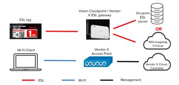
Customers must run ESL and wireless infrastructures in parallel and maintain hardware and software for both, increasing operational overhead.
