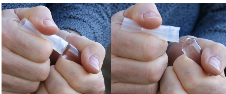
Figure 1: Open the ampoule. Leave the tubing on for protection.
