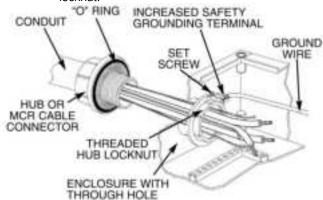
These locknuts must be bonded between each other and to the grounding system using jumper wires. After the entry hardware is installed, connect the appropriate conduit or cable.
