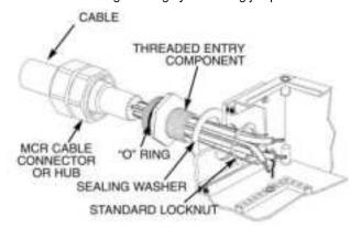
Refer to IOM sheet of cable connector for proper installation
