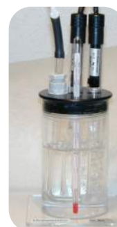
CAL300 with microsensors and bubbling with air.
