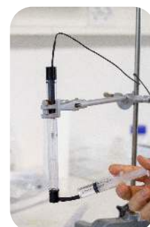
Injecting calibration liquid into protection tube using the calibration cap.
