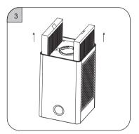
Remove the filter from the air purifier.
