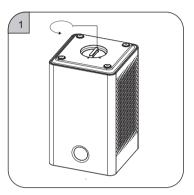
Make the product stand upside down and turn the knob on the base to open position according to the product's label.
