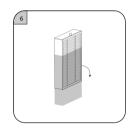
6. Remove the packing plastic bags of the new filters.
