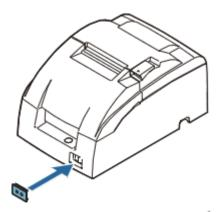
You can use the on/off switch cover provided to ensure that the switch is not operated unintentionally. To install, simply push the cover over the switch. If you want to turn the On/Off switch on or off with the cover attached, you can insert a thin object into one of the holes in the cover and use this to operate the switch.
