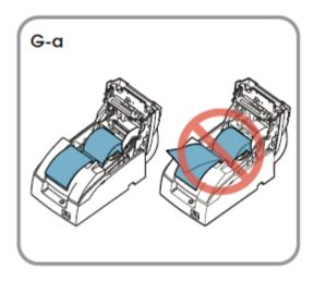
4. If you are not using a paper take-up reel, pull out a short piece of paper and close the paper roll cover; then tear off the paper using the manual paper cutter.
