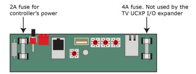
Symptoms of a blown fuse: Expander's power fuse - The expander's Pwr LED is not lit.
