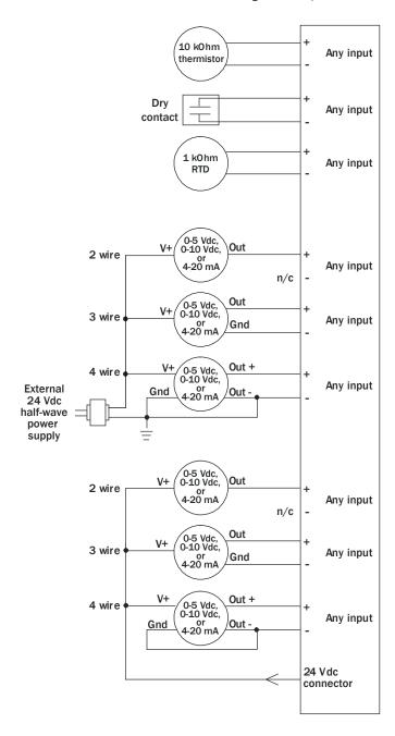
**NOTE** For a loop-powered 4-20 mA sensor, wire the sensor's positive terminal to the + terminal on the TV-UCXPIO48's **24 Vdc** connector. Wire the sensor's negative terminal to an input's + terminal.
