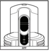
Slide switch to the bottom to turn off power To begin vacuuming in **Standard Mode**, slide switch to the desired setting.
