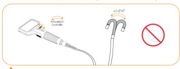
A Tips: To achieve the max articulation angle, the cable should not be coiled in a circle
