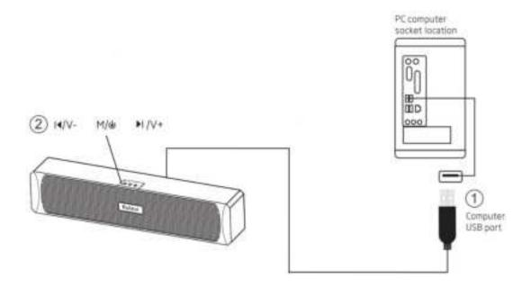
△ Single USB cable plug into computer USB port to ensure power supply.
