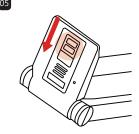
Remove the lens cover before operation
