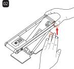
Hold the base plate and pull up from the middle hinge
