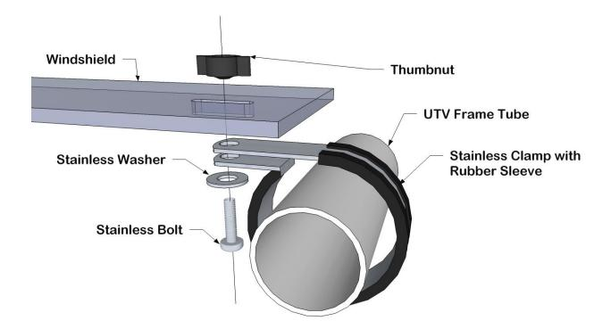
6. The four clamps that hold the windshield across the top use the large stainless and rubber washers to hold the windshield on. The inside part of it uses a small washer and a lock nut. The following photo shows how it should look.
