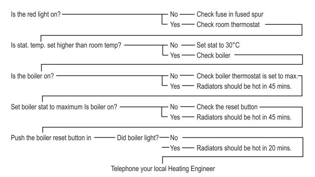
After the heating has come back on, return the programmer and other controls to the required settings.
