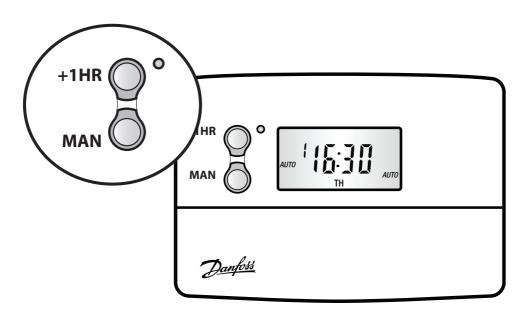
+1HR Pressing this button when the unit is in AUTO or ALLDAY mode will cause the system to remain on for an extra hour. If it is pressed while the programme is OFF the system will come on immediately for 1 hour then go off again. +1HR will be shown in the display.
