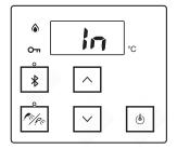
Controller alternates display between gas type and location.
