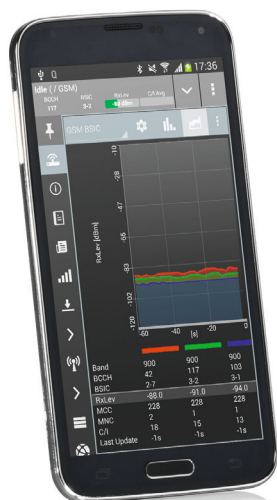
R&S®TSMA controlled from a SwissQual QualiPoc Android smartphone.
