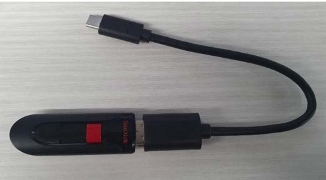
Figure 14. USB-C to USB adapter connections
