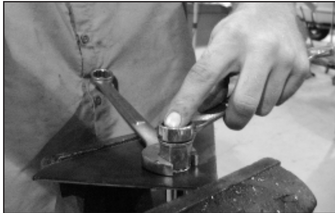
FIGURE 2 - 1/2" RIVET NUT SHOWN
