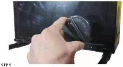
Insert the oil filter (M) into the oil inlet then cover it with the fuel cap (I)
