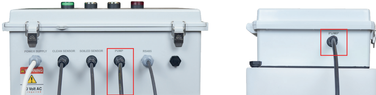
Figure 12 – Connection of the Water Pump Cable
