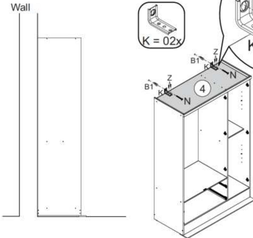
You will need a pencil to mark where you should drill the wall with a 3/8" drill bit to put in the hardware ( B1 )
