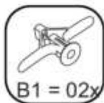
Put hardware (B1) in to the hole that you drilled on the wall
