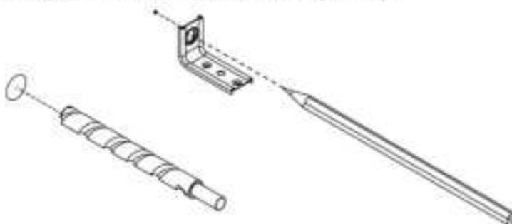
Use the 3/8 drill bit to drill the wall
