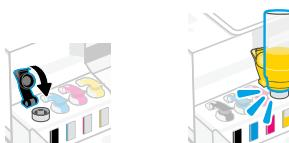
**EN** Open each tank cap and then fill all the tanks.
