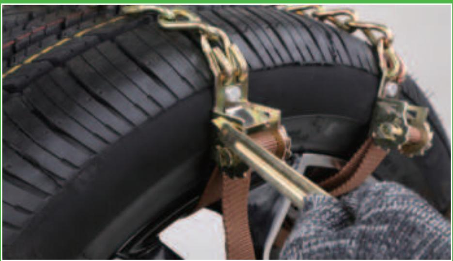
If you want to remove the chains, press the metal clasp and pull out the fastener.
