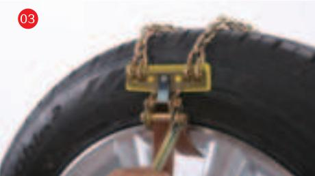
Rotate the shaft using the special wrench until it is tight.
