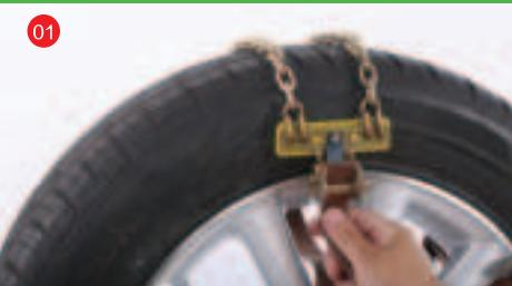
Pass the fastener through the first recess of the chain.
