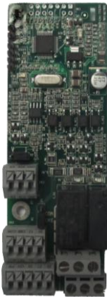
I/O expansion card 1 EC-IO501-00
