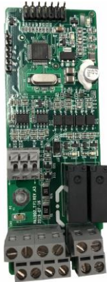
I/O expansion card 2 EC-IO502-00
