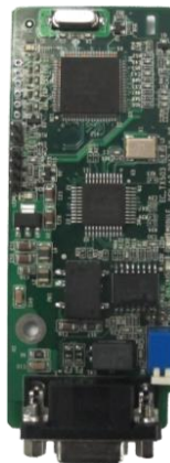
PROFIBUS-DP communication card EC-TX503
