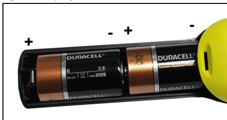
Figure 1 Properly installed alkaline batteries
