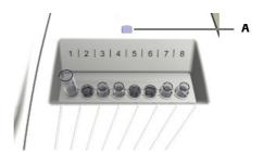
**A** Sample area LED. A green LED indicates that you should place a tube, a blinking yellow LED that you should keep clear of the sample area.
