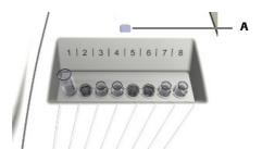
A The LED indicates that the transfer tower is approaching or that you should place a sample tube.
