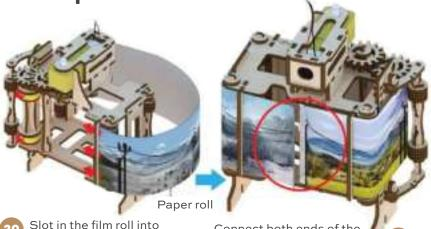
Slot in the film roll into the openings of part (47) from Step 23. Loop it into a circular direction as shown in the graphics.
