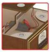
Insert the other sides of wires matching the black color wires to blue color switch and red color wires to yellow color switch. Once done, press down the switch to connect the wires.
