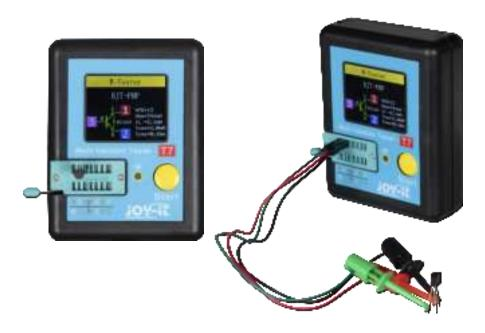
When you have connected your component, press down the lever and start the measurement with the start button.
