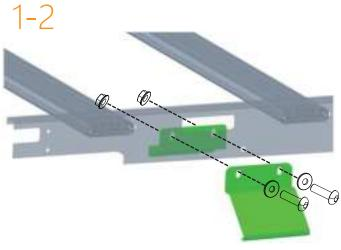
Mount the rear roof rack, ensuring the bracket screws remain adjustable.
