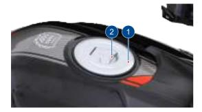
The fuel tank is not a measuring instrument and the capacity of the fuel tank may slightly vary from the indicated capacity. To avoid accumulation of water in the fuel tank, a small drain hole and a pipe is provided in the fuel tank lid cavity so that the water entering through the lid is drained out through the hose.
