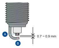
Visually inspect the spark plug gap. The gap should be 0.7 to 0.9 mm. If the gap is found to be more than the limit replace the spark plug with a new one.
