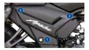
To assemble the cover frame back
