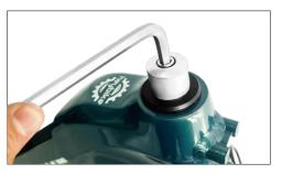
Locate the bike head part and using an Allen wrench, loosen the fastening screw. Then remove the washer.
