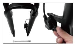
1 Locate the fork and remove the stud bolt fork protection. Remove the black retainer from the brake caliper.
