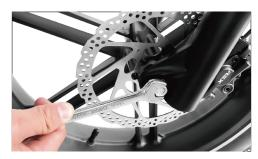
Completely feed the front wheel stud bolt through the front wheel center shaft, starting from the side with the brake disc. Firmly tighten the stud bolts.
