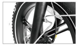
4 Using an Allen wrench, remove the two screws located on either side of the front fork, align the metal pieces from the fender with the holes, then return and tighten the screws.
