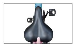
3 Adjust the seat and the head of the seat is parallel with the top tube.
