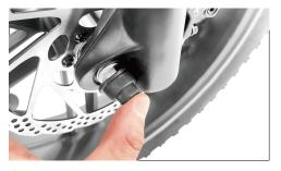
4 Place the front wheel screw covers onto both ends of the front wheel stud bolt.
