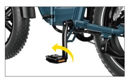
3 Thread the left pedal onto the left crank gently by hand, turning counter-clockwise. Then tighten the pedal with an wrench.
