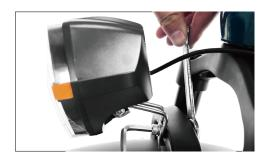
Using a wrench and Allen wrench, fasten the headlight and fenders above the front fork.
