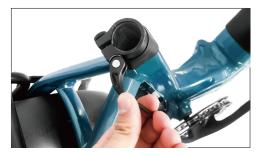
1 Open the quick release lever by swinging the lever open and outward fully.
