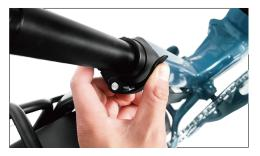
2 Move the seat up and down by sliding the seatpostin or out of the seat tube. DO NOT raise the seatpost beyond the minimum insertion marking etched into the seat post tube.
