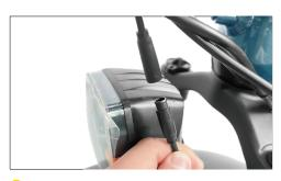
3 Connect the headlight power cable with the cable connected to the handlebar. Connect the display power cable with the handlebar cable.
