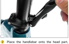
adjusting the handlebar angle to ensure it is properly aligned with the bike. Pull down on the quick-release lever and lower the handlebar.
