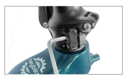
Using an Allen wrench, tighten the screws around the bike head part..
