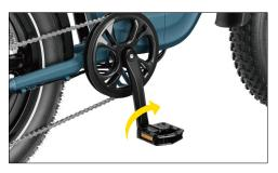
Thread the right pedal onto the right crank gently by hand, turning clockwise. Then tighten the pedal with an wrench.
