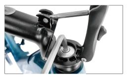
Using an Allen wrench, fully tighten the screw. Replace the handlebar to its upright position and engage the quick-release lever by lifting it up.
