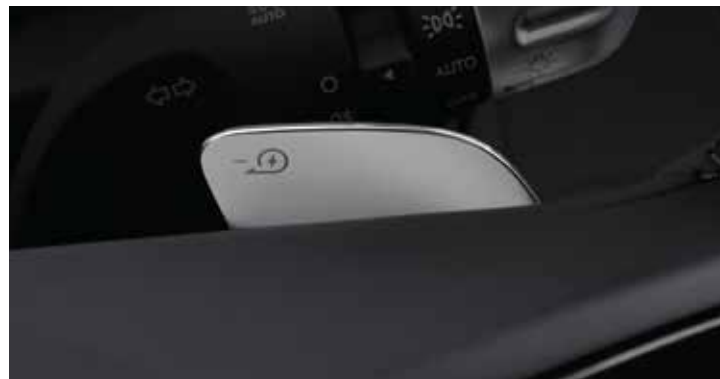
Paddle Shifter for Regenerative Braking
