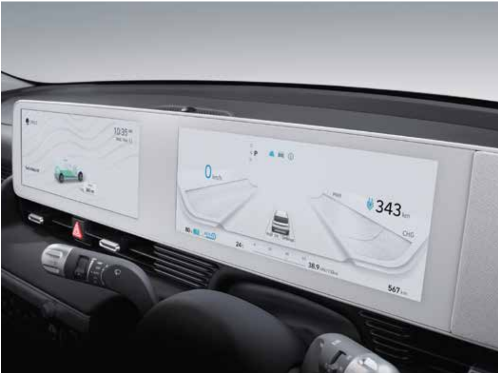
12.3" TFT LCD Cluster with integrated A/V System
