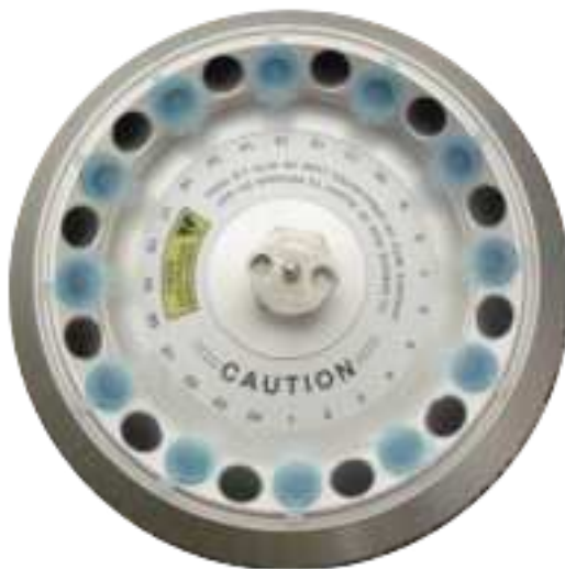
Figure 1. Loading the rotor to achieve balance.
