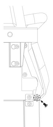
Install screw and tighten. (screw was removed in Step 13)
