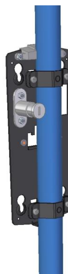
Figure 5: Mounting bracket attached to the pole
