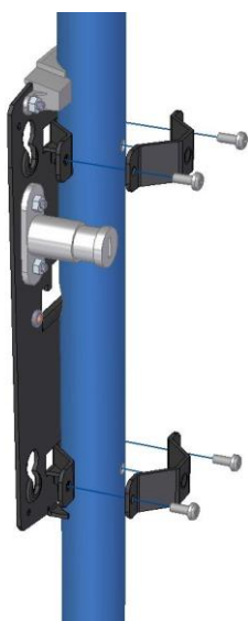
Figure 4: Attach the mounting bracket to the pole
