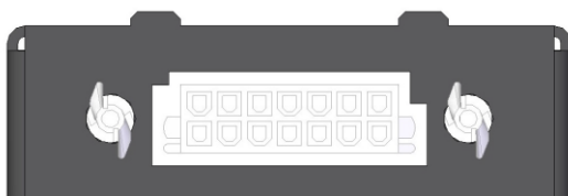
Figure 2: Connector block orientation
