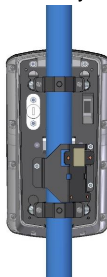
Figure 7: USB dongle bracket showing all fixings
